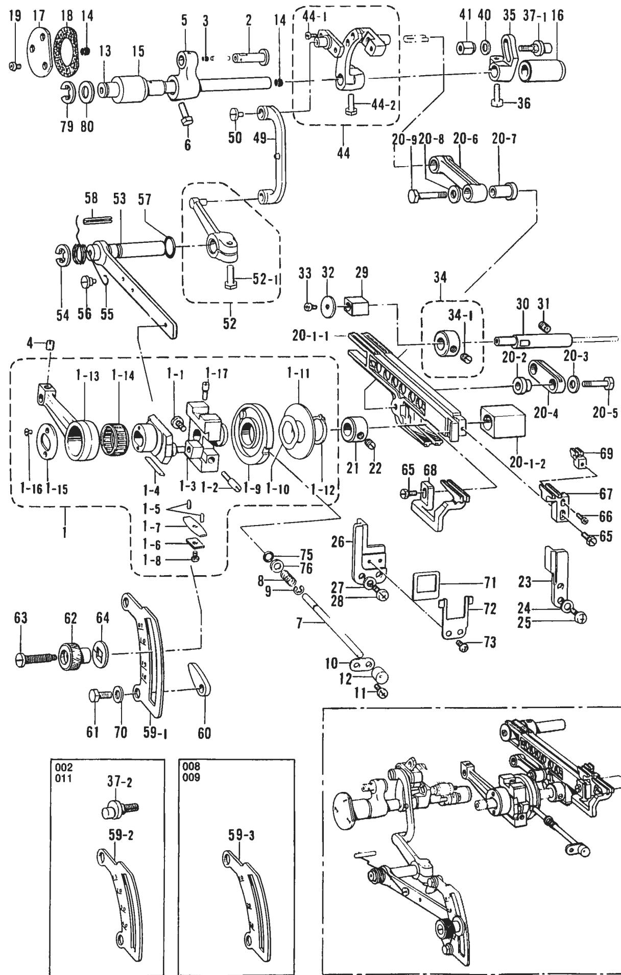
F. 送り関係/Feed mechanism/Transportvorrichtung/
