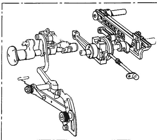
F. 送り関係/Feed mechanism/Transportvorrichtung/
